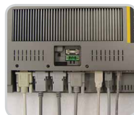
Downward I/O cabling
