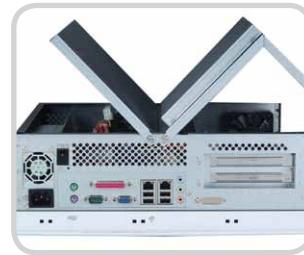
Gull-wing design, easy for installation & maintenance
