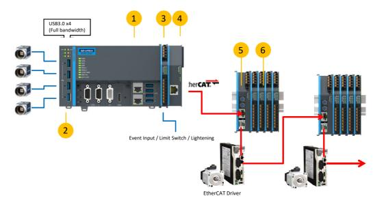
Figure 2.5 AMAX-5000 System Configuration for Motion + Vision Application
