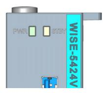
Figure 5.2 AMAX-5424V Module LED Indicator
