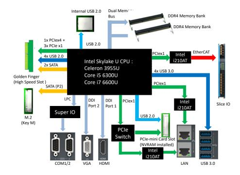
Figure 2.7 System Architecture of AMAX-5580
