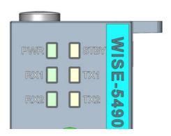
Figure 5.4 AMAX-5490 Module LED Indicator
