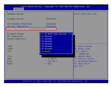
Figure 3.7 EC watch dog timer configuration in BIOS
