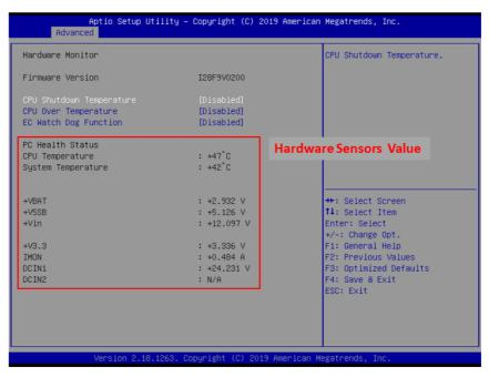
Figure 3.5 The Hardware Sensors Value showed in BIOS
