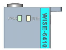
Figure 5.8 AMAX-5410 Module LED Indicator
