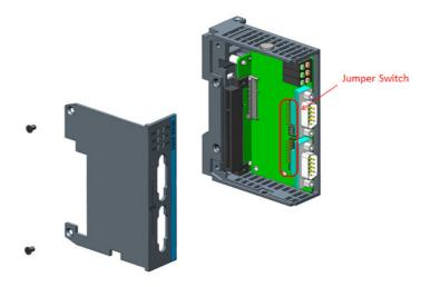
**Figure 5.5 Jumper Switch Location**
