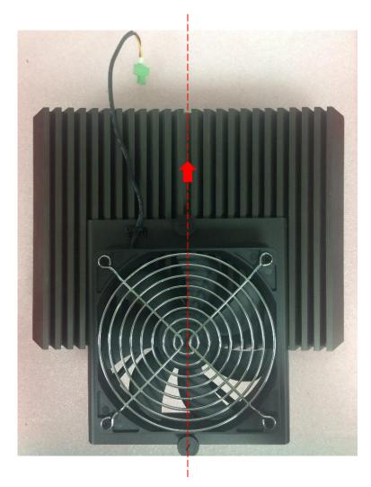
3. Move the fan to the center of chassis. Tighten the 2 screws marked on photo to secure it.
