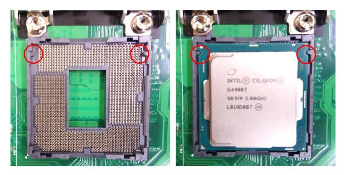
4. The notches of socket provide the space for fingers while lowering the CPU, hold the CPU by the edges toward the notches and insert the CPU gently.
