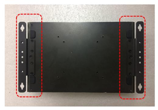
2. Fasten 2 DIN rail mounting clips to mounting brackets on both sides with provided 4 screws as illustrated.
