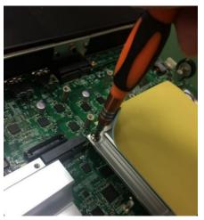
Note: Before assembling the system's chassis cover, please make sure the protective film on the Thermal Pad has been removed!
