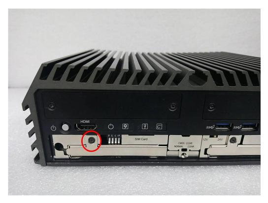
2. Pull the rotating arm and pull the HDD bracket out of system.
