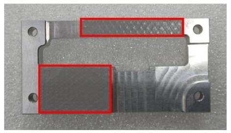
Note: Before putting on the thermal block (in the next step), please make sure the protective film on the Thermal Pad has been removed!
