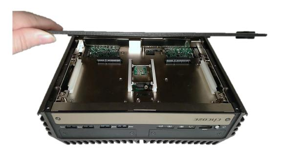
3. Loosen the 4 screws. Pull out 4 latches as marked on photo.
