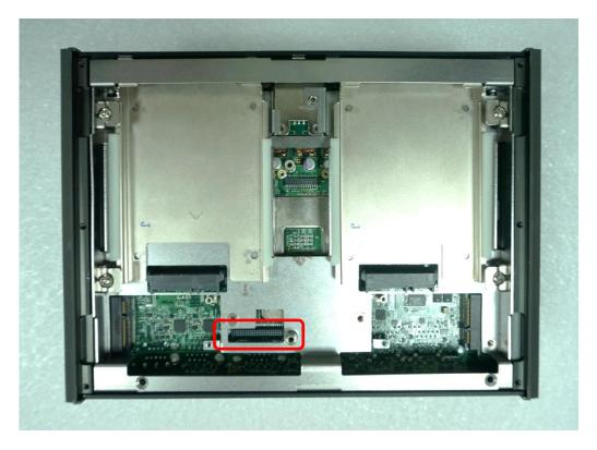
2. Loosen the 2 screws on rear bezel to remove the cover plate.
