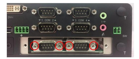
5. Attach the COM bracket. Fasten 2 screws and 4 D-Sub jack screws to fix it.
