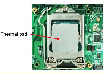
Note: Before putting on the thermal block (in the next step), please make sure the protective film on the Thermal Pad has been removed!
