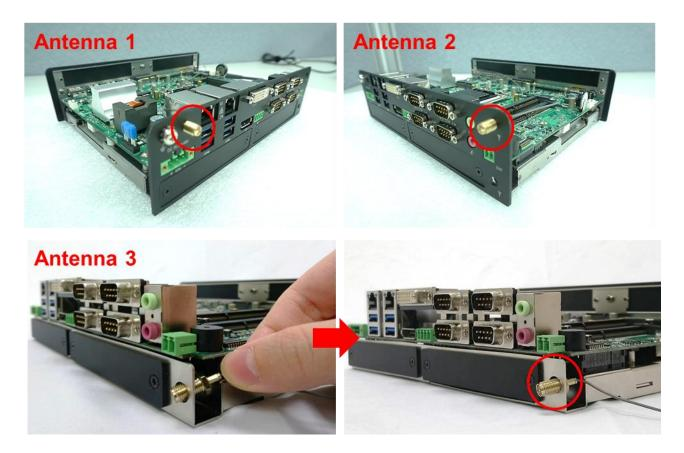
3. For antenna 1 and antenna 2, put on washer and fasten the nut with antenna jack. For antenna 3, put on rear panel back and fasten 10 D-Sub jack screws on it, and then put on washer and fasten the nut with antenna jack.
