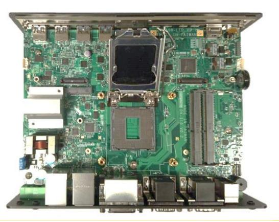
3. Align the notches on CPU with the alignment post on socket.
