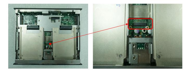
2. Fasten 1 copper pillar before insert IGN module.
