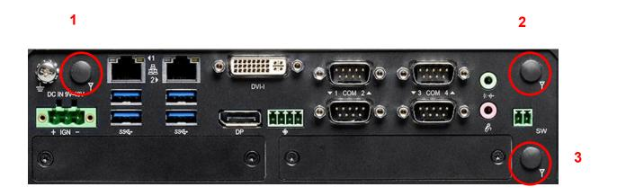
2. For antenna 1 and antenna 2, please penetrate the antenna jack through the hole at both sides as illustrated.
