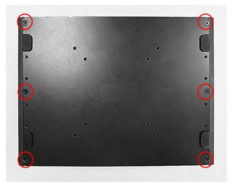
2. Remove the bottom cover from the chassis.
