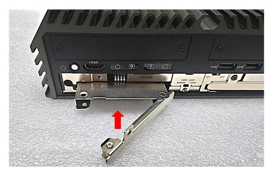
5. Place the rotating arm back and fasten the screw.
