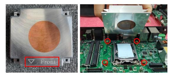
7. Flip the corner of thermal pad and fasten the heatsink with provided 4 screws.
