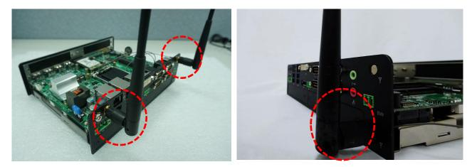
5. Attach the RF connector at another end of cable onto the module.
