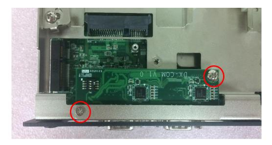
4. Loosen the 4 D-Sub jack screws as marked on photo.
