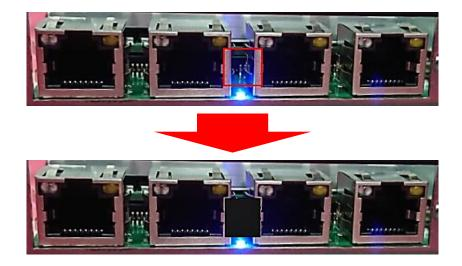
Insert the CMI-LAN module for DX-1100 vertically to the female connector (BTB\_FH2 or BTB\_FH4) on system's mainboard until it is connected firmly, and fasten 4 copper pillars to fix it. (CMI-M12LAN module is taken as the installation example in this chapter)
