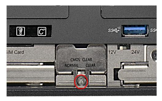
2. Pull out the CMOS battery bracket with assistance of a tweezer.
