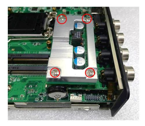
8. Paste the last thermal pad onto the heatsink carefully.
