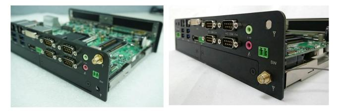
4. Assemble the antenna and antenna jack together.
