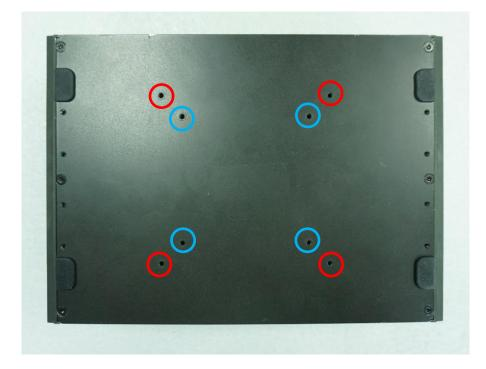
The following picture illustrates the installation of DX-1100 series on a VESA stand. Align the 4 screw holes of VESA stand with the screw holes on bottom side of system. Fasten 4 screws to fix it.
