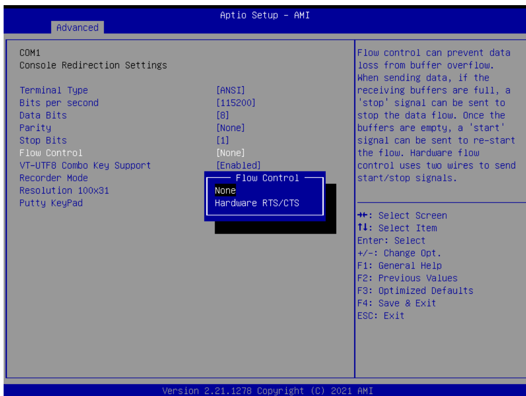
Figure 3.26 Flow Control Settings
