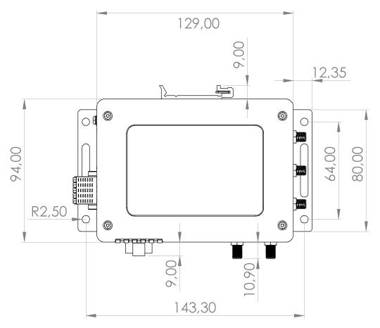
Figure 8: Basic dimensions of the router box
