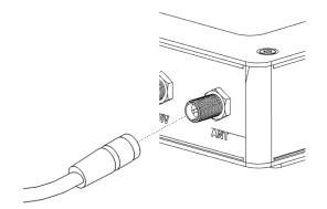
Figure 17: Connecting the antenna
