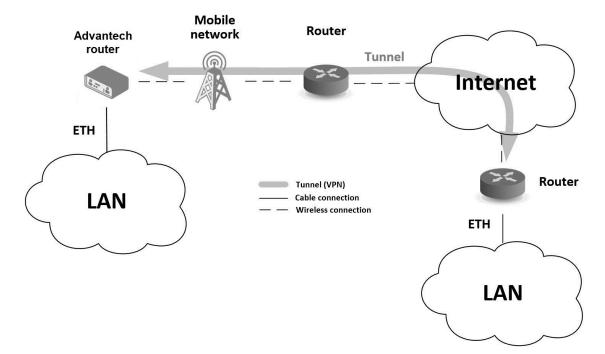
Figure 3: Using VPN tunnel
