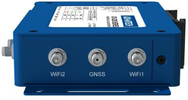
Figure 22: The right panel of the router
