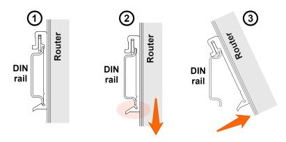
Figure 11: Removing from the DIN rail
