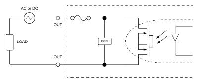
Figure 22: Binary output connection
