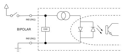
Figure 21: Binary inputs connection
