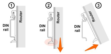
Figure 9: Removal from the DIN rail
