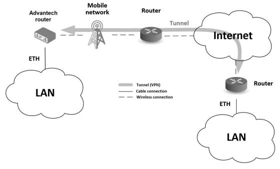
Figure 3: Using a VPN tunnel
