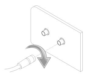
Figure 19: Connecting the antenna
