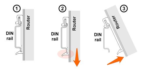
Figure 14: Removal from the DIN rail
