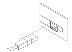
Figure 22: Connection of Ethernet cable
