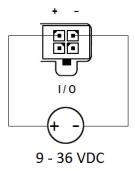
Figure 17: Circuit example – connection of power supply
